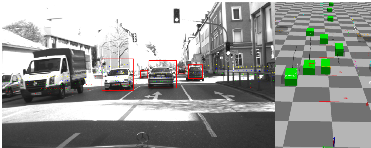
Fig. 5. Snapshot of the tracking results using the LMB filter in an urban scenario: On the left side, the video image and the object hypotheses of the video detector are shown. On the right side, the obtained tracks for the scene are illustrated using green boxes and the black lines represent the trajectories of their motion (relative to the ego vehicle).
